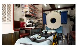
The unit is a specially modified ambulance with a CT scanner onboard
